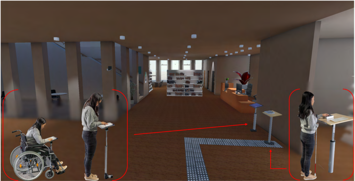
Figure 1: Photo montage of the environment modeled in VR using BIM data and the real prototypes: The left table, adjustable in height and inclinable, is designed for wheelchair users and general sighted users and holds an audiovisual display. The right table is fixed in height and inclination and holds a tactile tablet designed for blind people.
